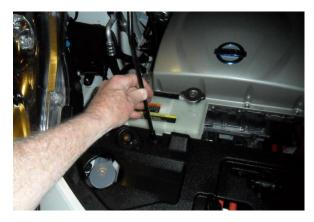
Ensure that the hood support rod is securely in the correct hole.
